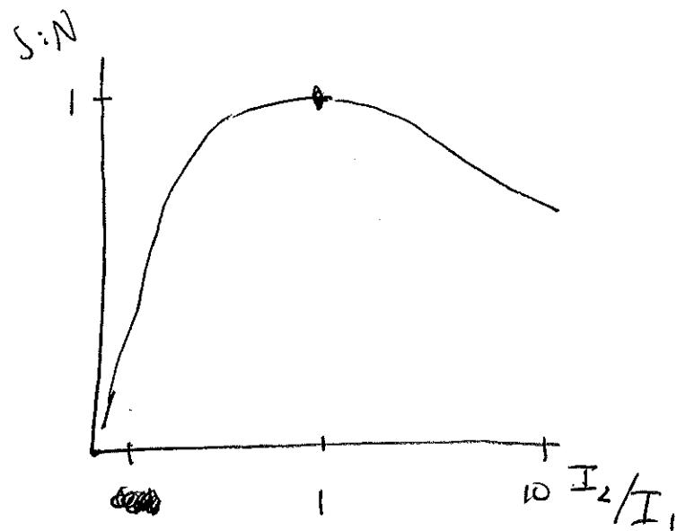
Signal to noise is maximum for  $I_2 = I_1$ .
